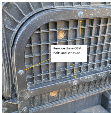
FIG 3 - Remove OEM Bolts using a T25 Torx
