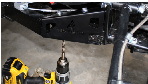
FIG 1 - Use 7/16" Drill Bit to drill holes in bottom of frame using Bracket (1) as template
