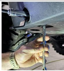
Next, remove all of the oem torx screws from the tops of the door sills and along the bottom at the skid plate. See below.
