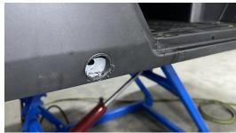
Next, insert the mount bracket into the hole, the the M8 x 55mm Hex Head Bolt, then fasten with a M8 Locknut from underneath the unit. There will be an access pocket in the skid plate that allows access to the back side of the frame rail. Tighten the bolt/nut up just enough to remove most of the slack, but leave loose until everything is mounted.
