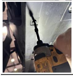
Next, place to bottom of the nerf rail up into place and loosely fasten with the M6 x 30mm screws and the M8 x 20mm button head screws. The M6 x 30mm screws will replace the oem torx screws that you previously removed along the bottom of the unit. The M8 screws will go up through the bottom of the nerf rail, through the mount brackets, and fasten with an M8 flanged locknut. See below
