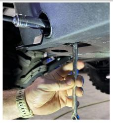
Next, remove all of the oem torx screws from the tops of the door sills and along the bottom of the rocker panel. See below.
