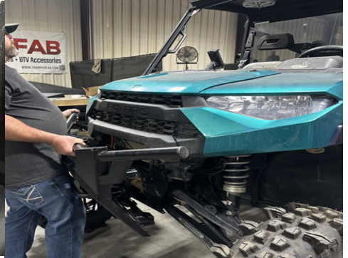
FIG 2 - Remove OEM Bumper
