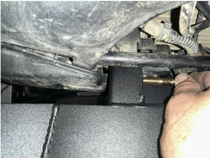
FIG 7 - Loosely fasten bumper to upper mounts using M10 x 60mm Flange Head Bolts (B)
