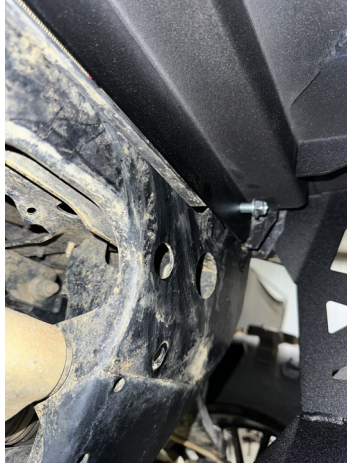
FIG 8 - Loosley fasten center mount using bolts (A) and nuts (C)
