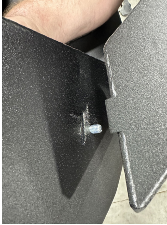
FIG 6 - Install Bull Bar using 13mm Wrench
