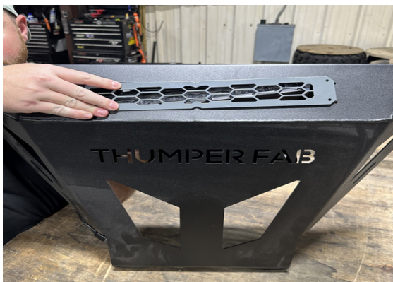
FIG 4 - Install Light Bar Cover using 9/64" Allen and 11/32" Wrench
