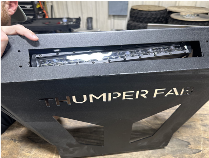
FIG 3 - If light bar was purchased, install using tools and hardware provided in light bar box
