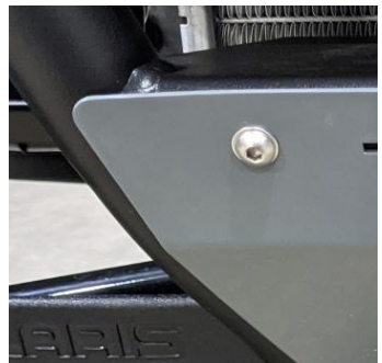
FIG 5 - Install Skid Plate 5/32" Allen, 7/16" Socket
