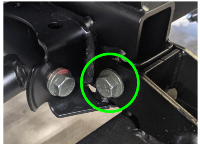
FIG 4 - Lower Side Bolt (SP 570) - 13mm
