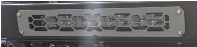
FIG 7 - Install Light Bar Cover - 9/64" Allen
