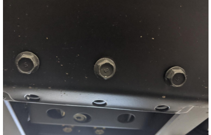
FIG 2 - Lower Bolts (500/570) - 13mm
