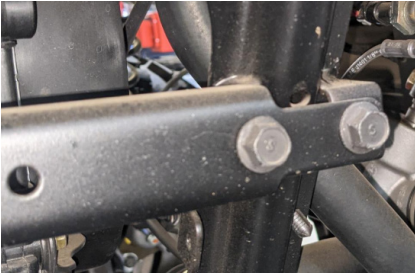
FIG 1 - Side Bolts (500/570) - 13mm
