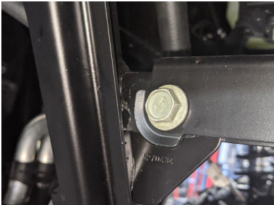
FIG 3 - Upper Side Bolt (SP 570)- 13mm
