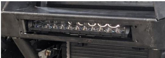
FIG 6 - Mount Light Bar
