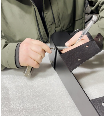
FIG 1 - Fasten Front Fender Flares together
