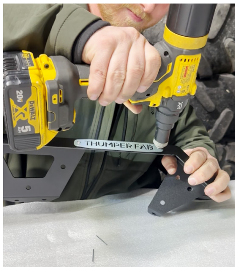
FIG 4 - Fasten Logo Plates to Rear Upper Fender Flares
