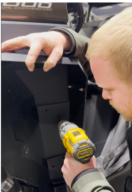
FIG 3 - Drill Holes using 5/16" Drill Bit
