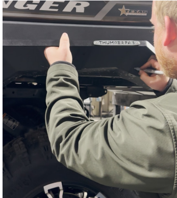
FIG 5 - Use Rear Fender Flares as a template to drill holes
