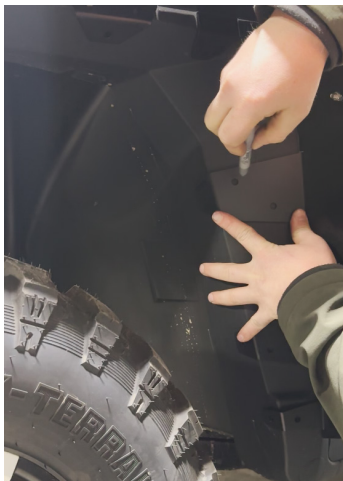
FIG 2 - Use Front Fender Flare as a template to mark and drill holes
