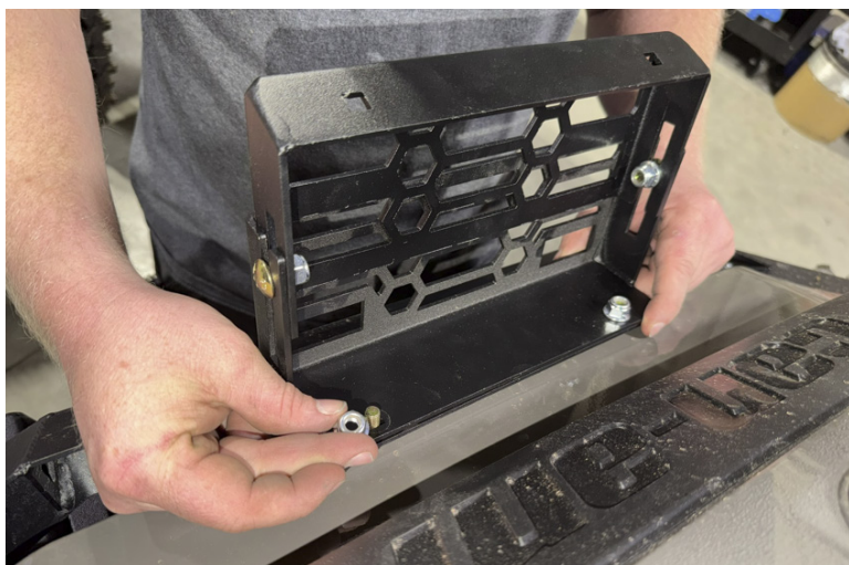
FIG 11 - Fasten TF Bumper Mount to Bumper Mount Bracket assembly
