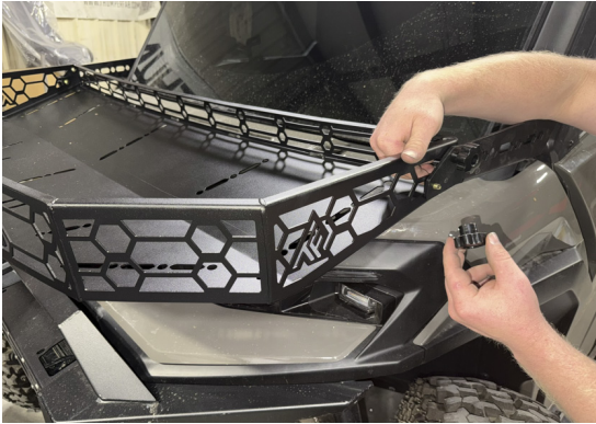
FIG 12 - Fasten Main Basket to rear Mount Brackets
