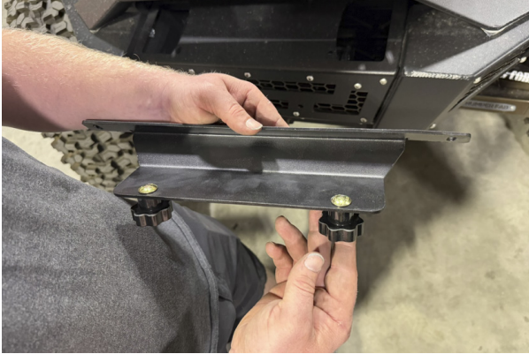
FIG 8 - Use plastic knobs to hold carriage bolts to TF Bumper Mount
