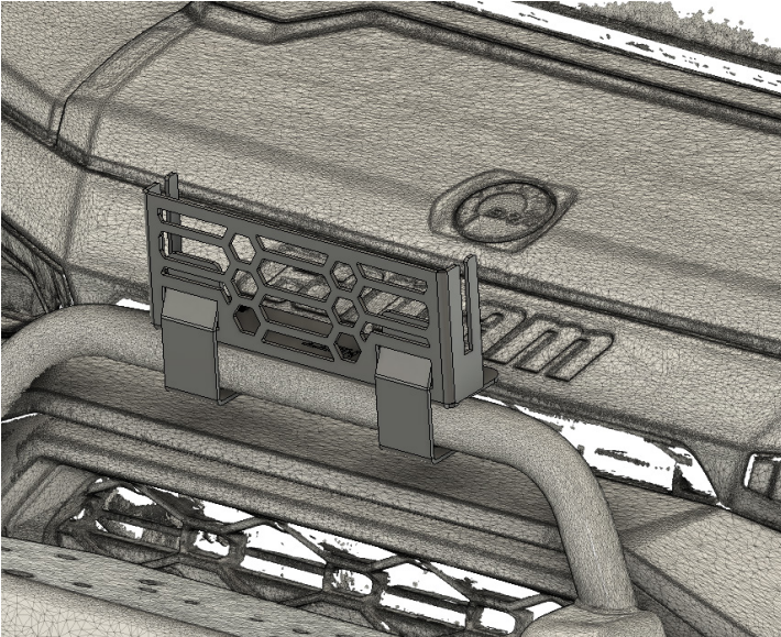
FIG 5 - Slot OEM Bumper Mounts into Bumper Mount Outer Bracket
