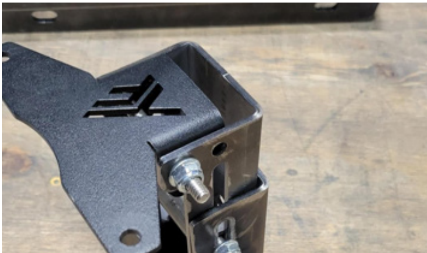
FIG 4 - Fasten Pivoting Attachment Plate to Bed Rail Adjustment Plate using 7/16" Socket and 7/16" Wrench
