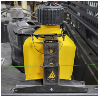
FIG 6 - Adjust height of Jug Holder to grab jug neck. Tighten using 7/16" Wrench
