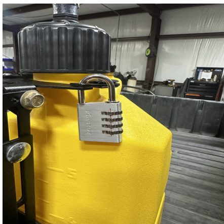
FIG 12 - Lock can be used in place of Button Lock Pin (G)
