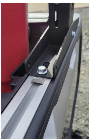
FIG 15 - Fasten Jug mount to rail using 12mm Socket
