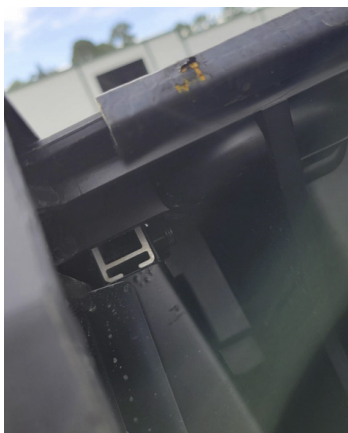
FIG 13 & FIG 14 - Insert 2 x Lock and Ride Max Fasteners (L) into rail
