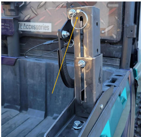
FIG 8 - Rotate Pivoting Attachment Plate down and lock using Ring Lock Pin (F)
