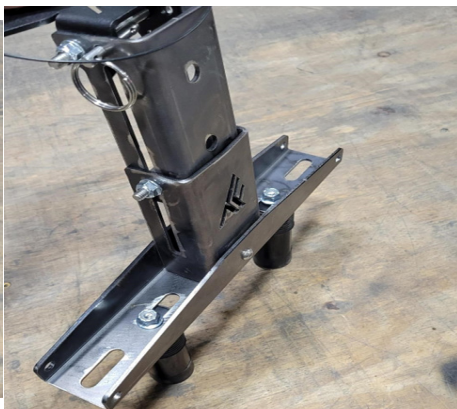
FIG 9 & FIG 10 - Loosley fasten lock and ride fasteners to jug mount assembly
