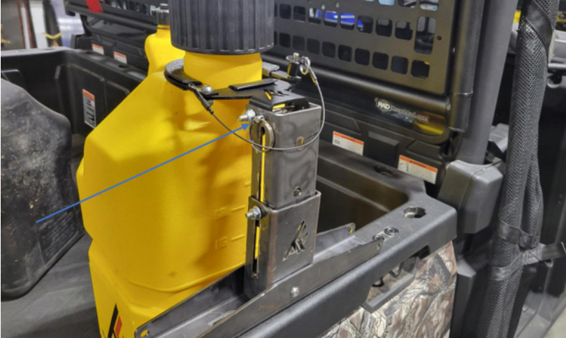
FIG 7 - Install Ring Lock Pin (F) to lock Pivoting Attachment Plate (5)
