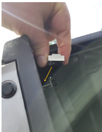
FIG 13 & FIG 14 - Insert 2 x Lock and Ride Max Fasteners (L) into rail
