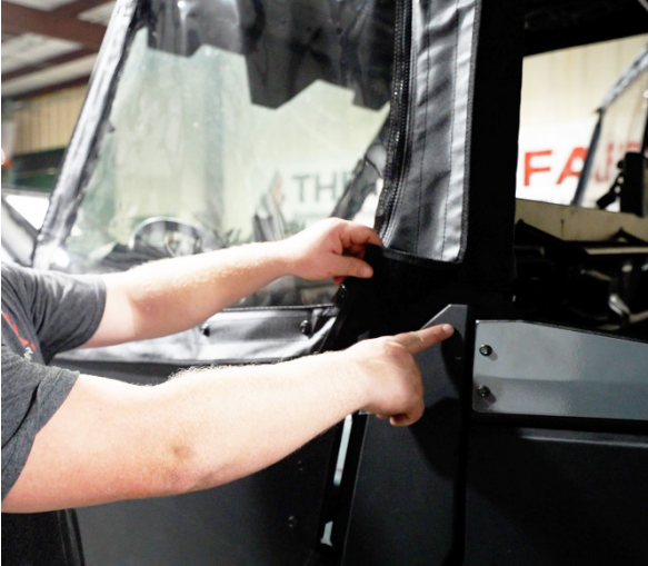
FIG 16 - Apply Velcro Tape to area shown and Velcro lower corner of front door vinyl to chassis
