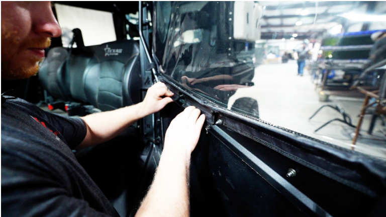
FIG 9 - Fasten Vinyl to the inside of Upper Door Frame using Velcro Tape
