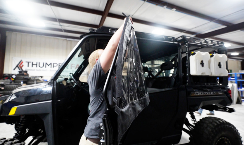
FIG 6 - Fasten Vinyl to the Upper Door Frame using the Velcro straps
