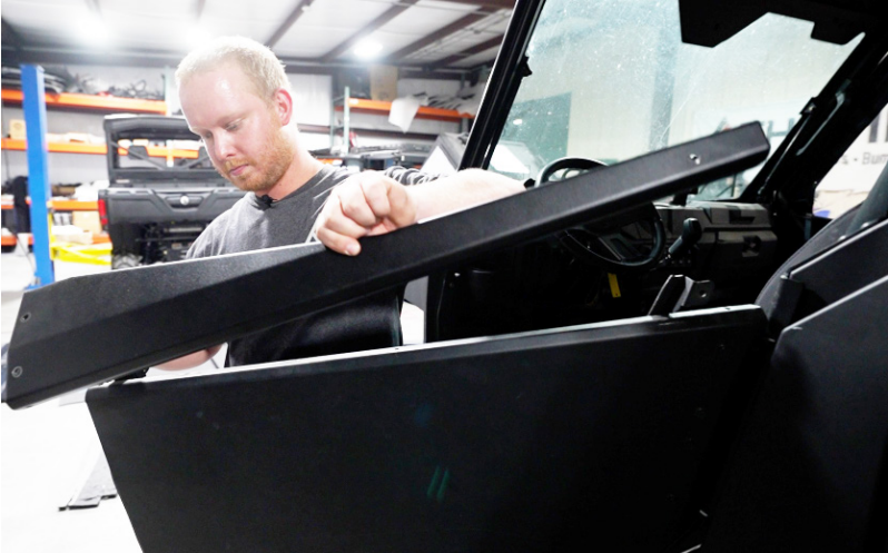
FIG 1 - Remove Half Door Upper Skins using 3/8" Socket and 7/16" Wrench
