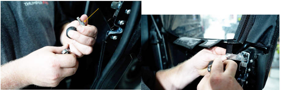
FIG 17 - Slide Spacer over existing hex bolt FIG 18 - Tighten latch bracket assembly using 10mm Wrench
