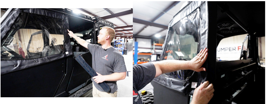
FIG 14 - Velcro Center Panel to B-Pillar of roll cage
