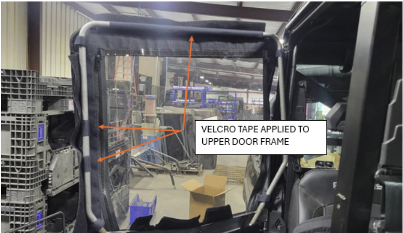
FIG 5 - Velcro Tape Applied at specified locations
