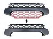
Mount the base plate to the Ranger Chassis with 4 of the original bolts, then tighten with sufficient torque. If your model does not have all needed hardware, use included 10 mm hardware.
