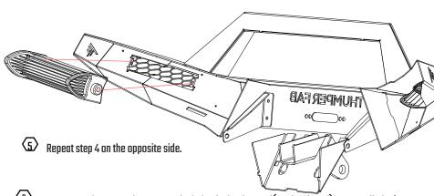
Mount your Thumper Fab Bumper. The holes facing forward(marked in red) use supplied 5/16" hardware. The holes facing the side use two of the stock bolts that you should have remaining from removing the stock bumper.
