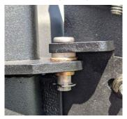
For the bottom connection, the order from top to bottom should be *clevis pin*  $\rightarrow$  *bike-side bracket*  $\rightarrow$  *white spacer*  $\rightarrow$  *bushing*  $\rightarrow$  *door-side bracket*  $\rightarrow$  *retaining ring.* See image below.
