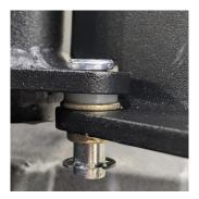
Remove the T-40 hardware pictured on the stock side plastic trim piece an then use the removed hardware to install the hinge assembly over the trim. Attach hinge assembly to the front and rear hinge brackets with 5/16" bolt (*F*), nut (*H*), and flat washer (*G*) using 1/2" wrenches. The washer should be placed on the bolt side. *Tighten firmly.*
