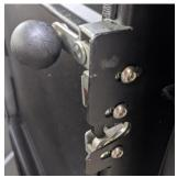
2. Lift door and attempt to latch the door to the striker pin. As you push the door closed, you should hear two clicks from the latch. If the latch is fully engaged, the bottom of the black locking mechanism should be parallel with the rest of the latch as seen below. If the latch will not fully engage with the striker pin, you may need to adjust by repositioning the latch by adjusting the 3 bolts in step one. If it still will not engage, you may need to adjust the positioning of the latch pins.
