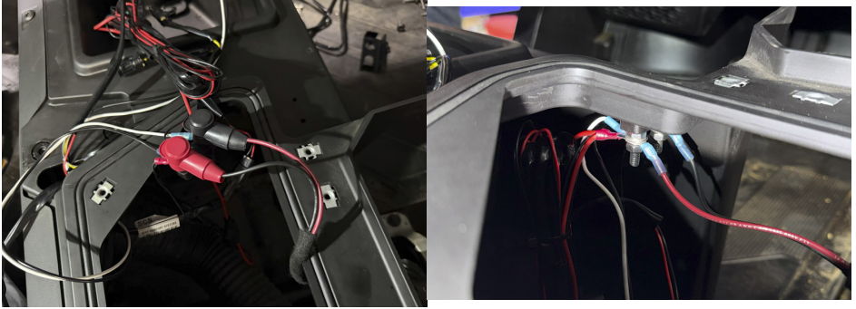
FIG 36 & FIG 37 - Fasten junction block to inside of under seat cubby
