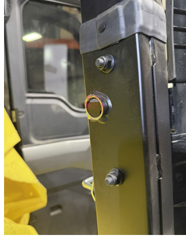
FIG 12 & 13 - Cut the harness tube and seat belt mount as close to the B-Pillar using a reciprocating saw
