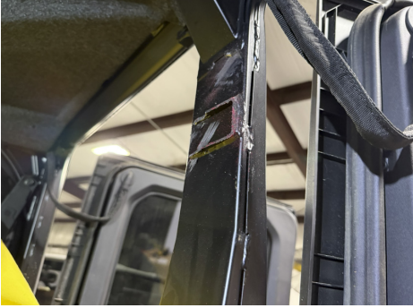
FIG 12 & 13 - Cut the harness tube and seat belt mount as close to the B-Pillar using a reciprocating saw
