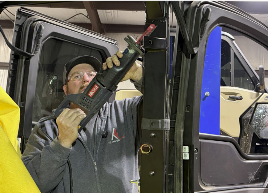
FIG 11 - Cut the upper seat belt mounts at the B-Pillar
