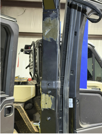
FIG 16 & FIG 17 - Use touch up paint on the bare metal locations of the B-Pillar
