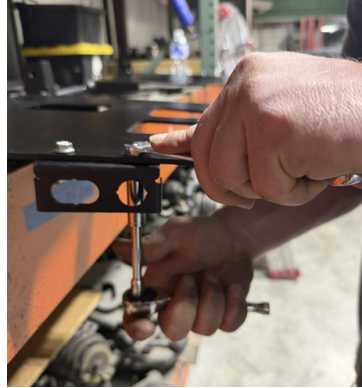
FIG 40 & FIG 41 - Plug the harness into the pulse bar and fasten the seat switch panel to the seat mount frame
