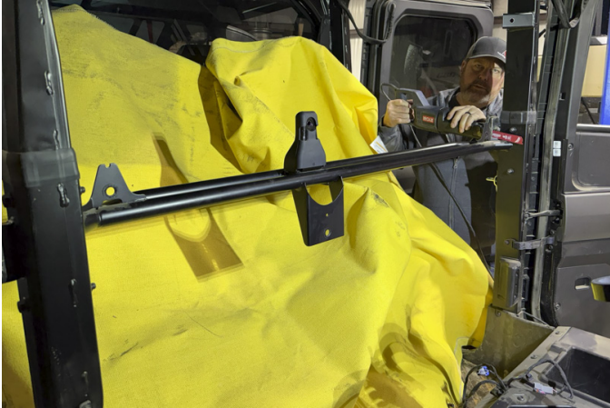
FIG 10 - Cut the harness tube at the B-Pillar using a reciprocating saw
