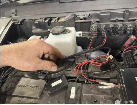
FIG 40 & FIG 41 - Plug the harness into the pulse bar and fasten the seat switch panel to the seat mount frame
