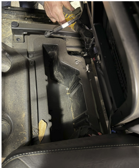
FIG 2 - Remove remaining seat frame OEM mounting bolts under the front seat
