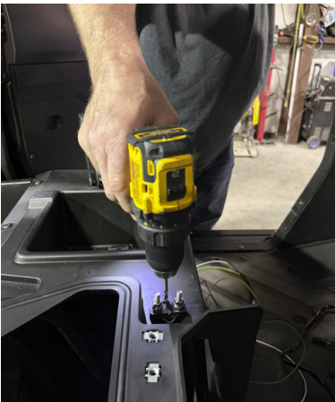
FIG 34 & FIG 35 - Drill holes for junction block and attach seat heater and optionally electric slider harness (if slider option was selected)
