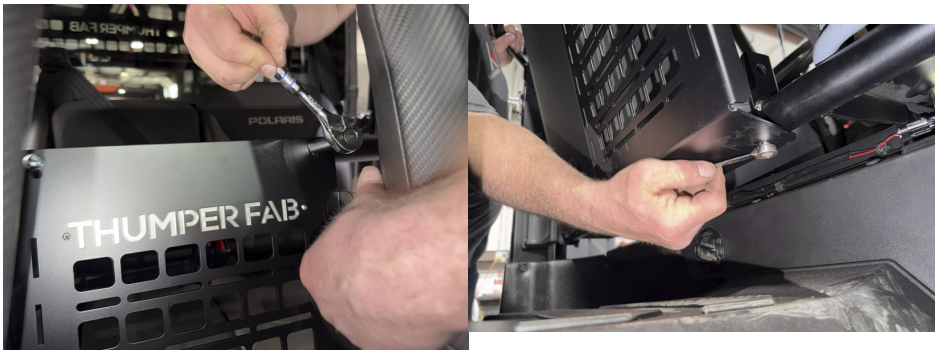
FIG 59 & 60 - Fasten the center console main mount to the harness bar and the seat frame
