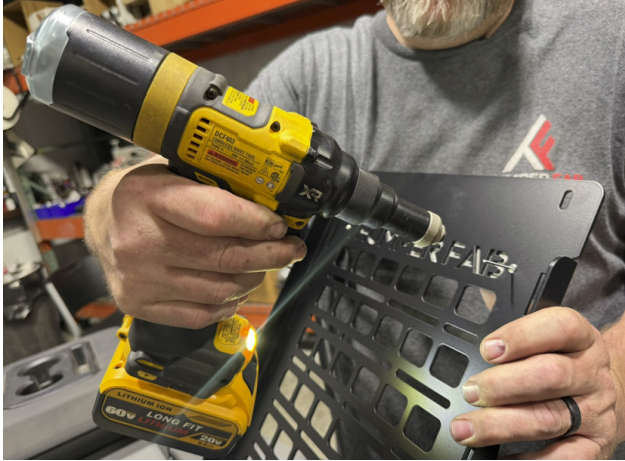
FIG 58 - Mount the backing plate to the center console main mount
