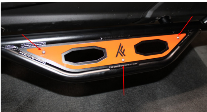
FIG 8 - Install Accent Panels (3/32" Allen Wrench)
