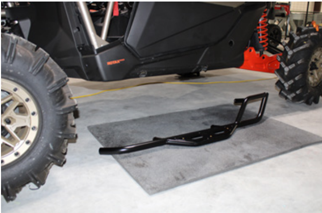
FIG 4 - Stage for Nerf Rail Installation
