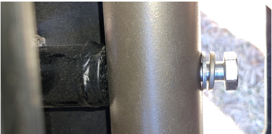
FIG 5 - Bolt and Washer Sequence (17mm Wrench)
