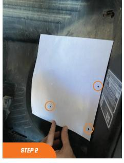
Align the template with the factory hole locations then mark the additional hole location with a scribe tool.
