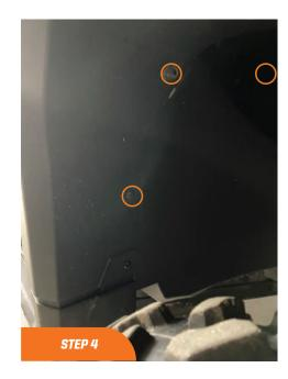
Once all 3 holes are aligned, use the (2) two M6x20 bolts and washers in the factory hole locations and (1) one M6x16 bolt and washer in the drilled hole location to secure the pod to the vehicle. Hand tighten all bolts.
