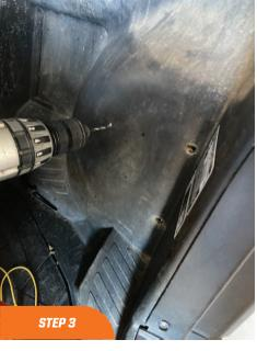
Drill a 5/16" hole in the marked location.
