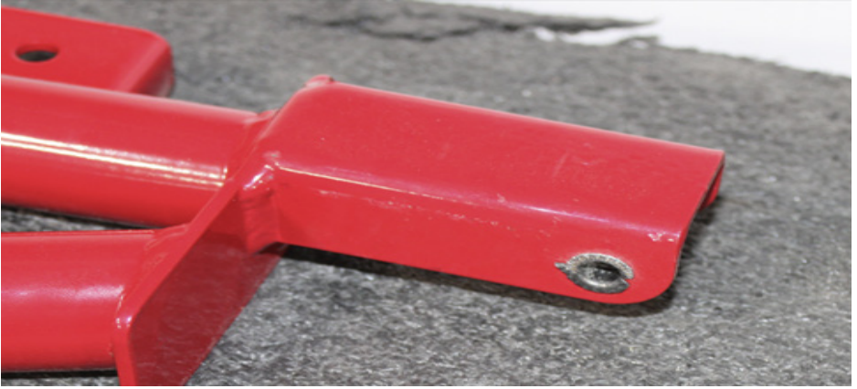
FIG 9 - Install Rear Door Hinge OEM Bushings
