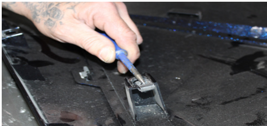
FIG 15 - Remove OEM barrel clip nuts using small punch
