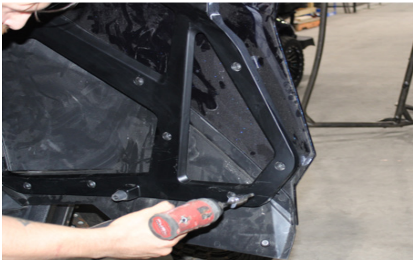
FIG 3 - Remove Rear Door Skin with T40 Torx
