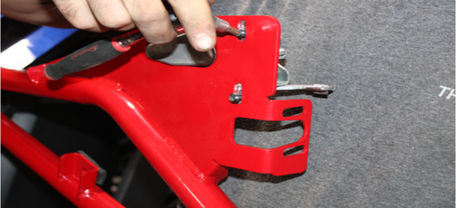
FIG 13 - Install Oem Door Release Button using T25 Torx
