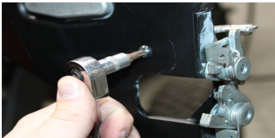
FIG 4 - Remove Rear Door Latch Button using T25 Torx
