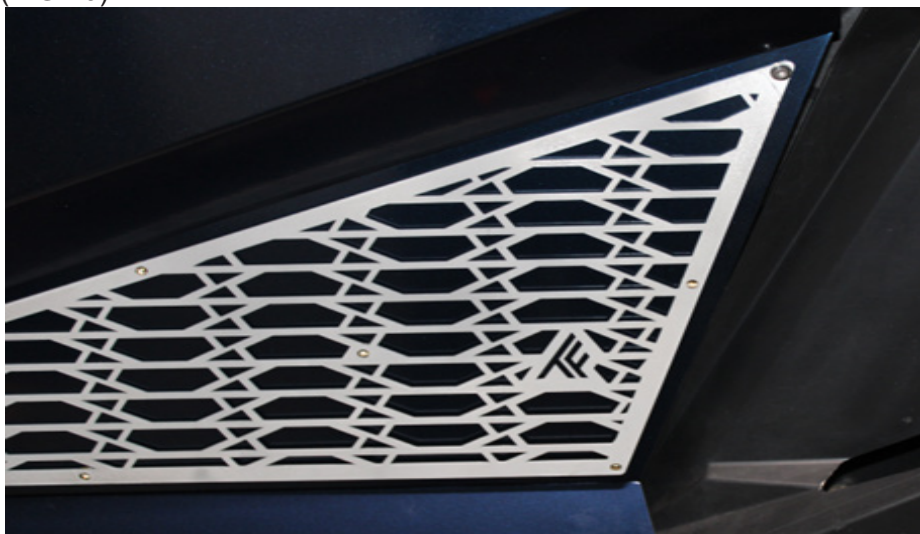
FIG 20 - Install front and rear accent panels using 5/32" Allen and 7/16" Socket
