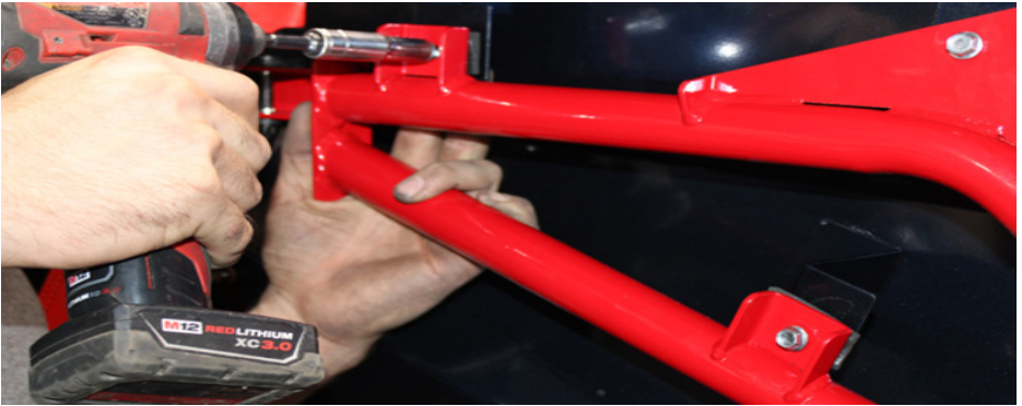
FIG 17 - Install rear door skin using 10mm Socket
