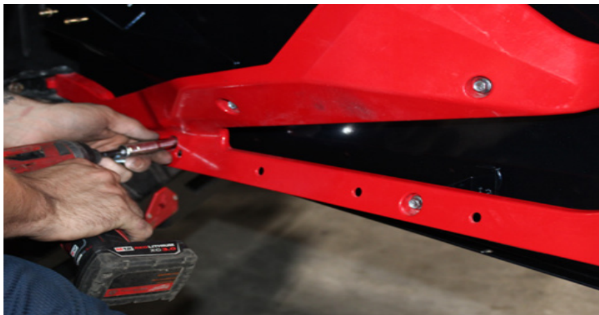
FIG 19 - Install front door skin using 10mm Socket
