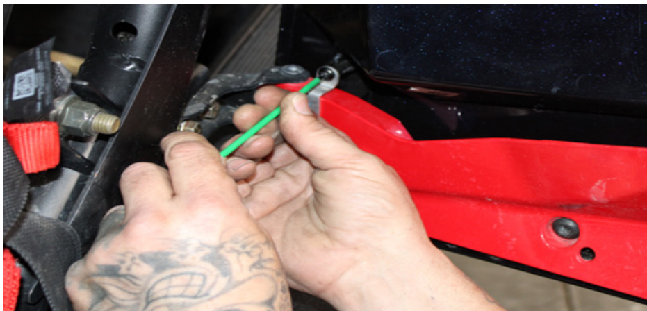
FIG 1 - Remove Door Strap with T25 Torx
