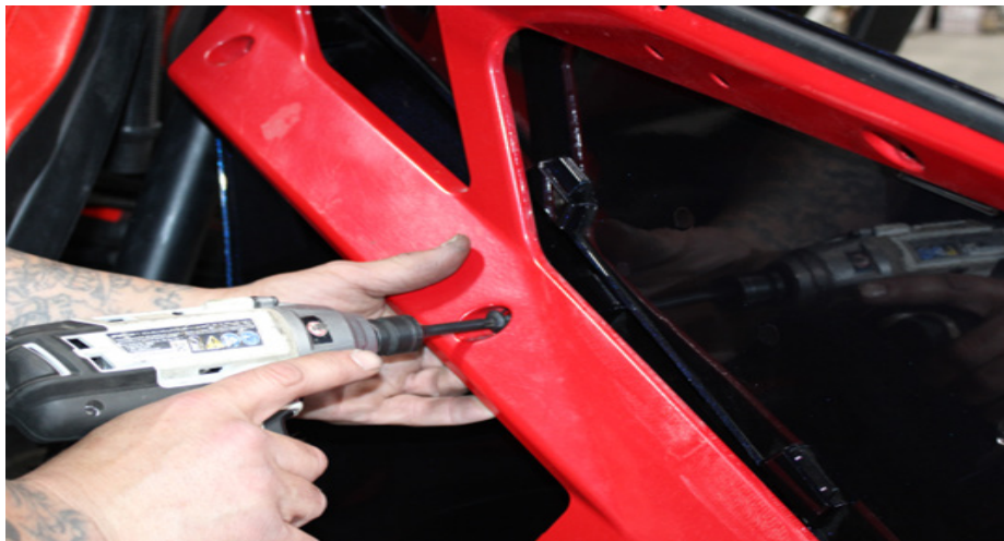
FIG 2 - Remove Front Door Skin using T40 Torx
