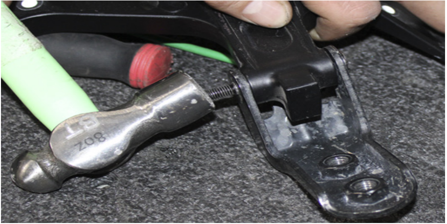
FIG 7 - Remove Rear Door Hinge Pins using a Dead Blow Hammer
