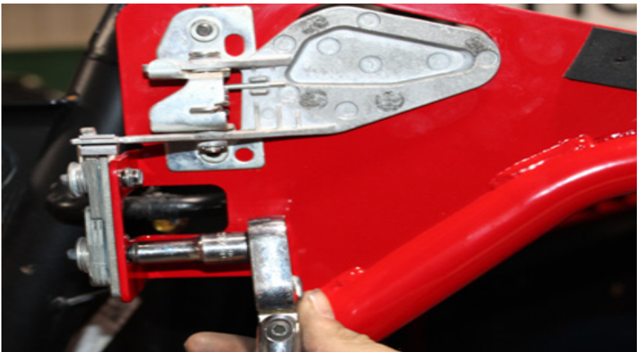
FIG 14 - Install latch onto frame using 8mm Socket
