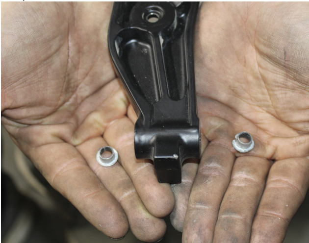
FIG 8 - Remove Door Bushings using a small Flathead
