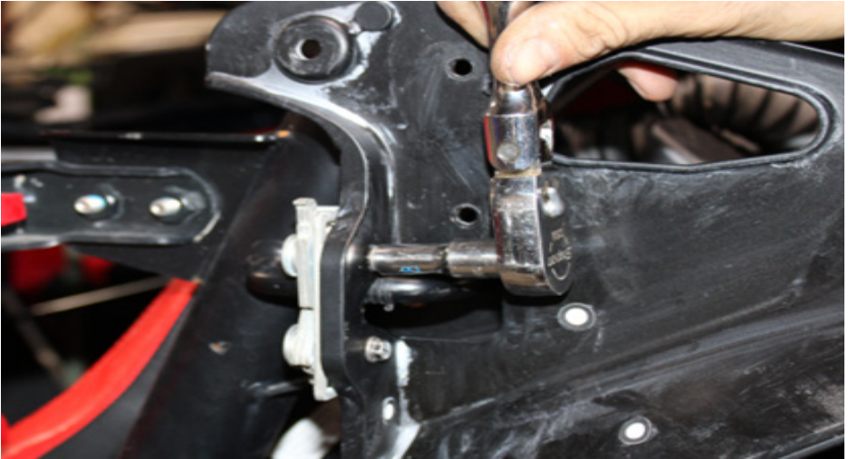
FIG 5 - Remove Rear Door Latch using an 8mm Socket
