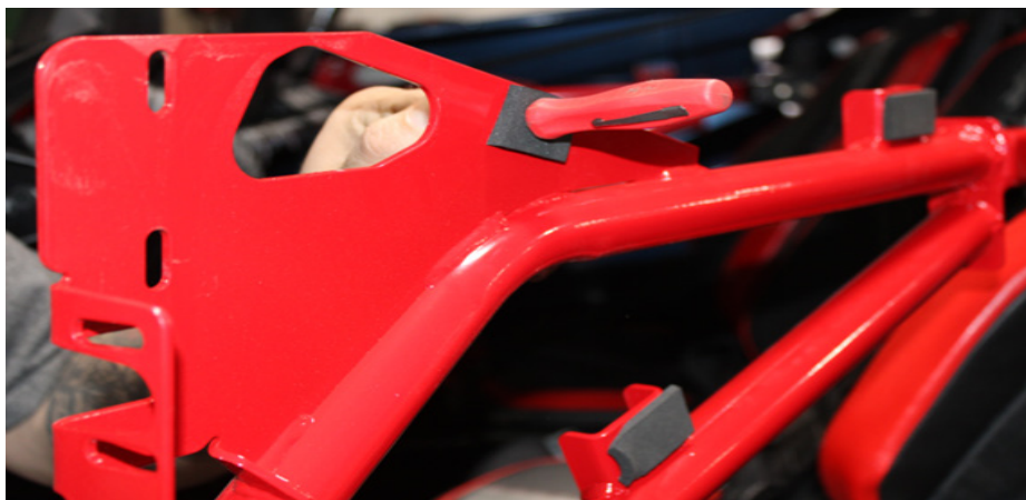
FIG 12 - Apply foam to mounting positions, poke hole with Screwdriver
