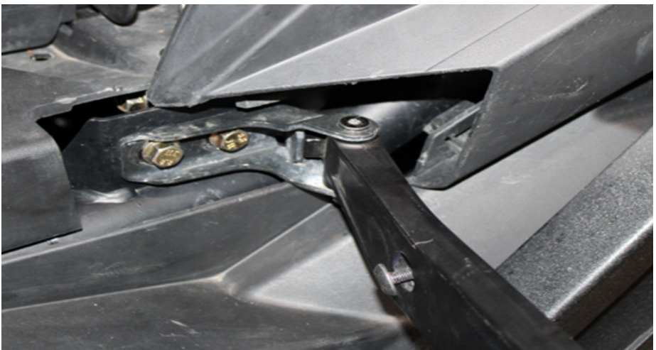
FIG 6 - Remove Rear Door Hinges and Frame using 13mm Socket
