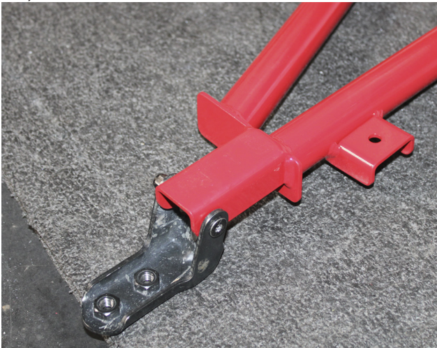
FIG 10 - Install OEM hinges using 8mm Socket
