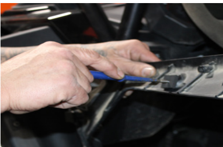
FIG 5 - Install noise dampening foam over mount holes of door frame
