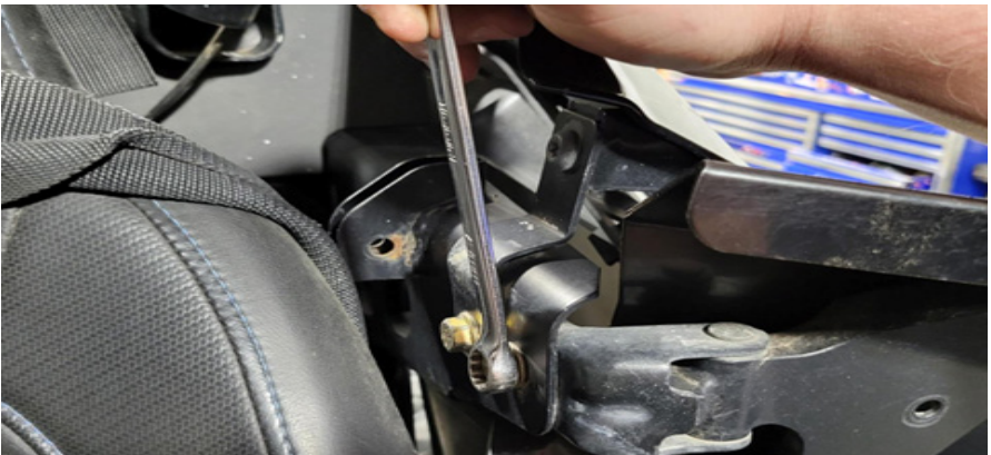
FIG 9 - Adjust OEM hinges as needed using 13mm Wrench
