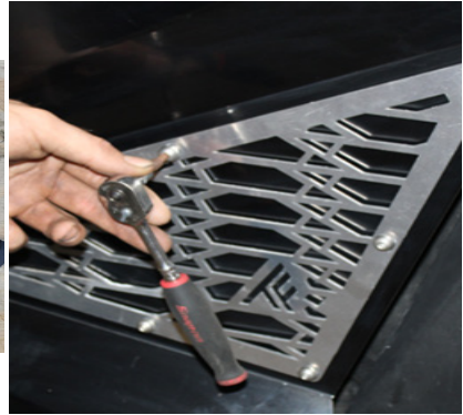
FIG 8 - Install accent panels using 5/32" allen
