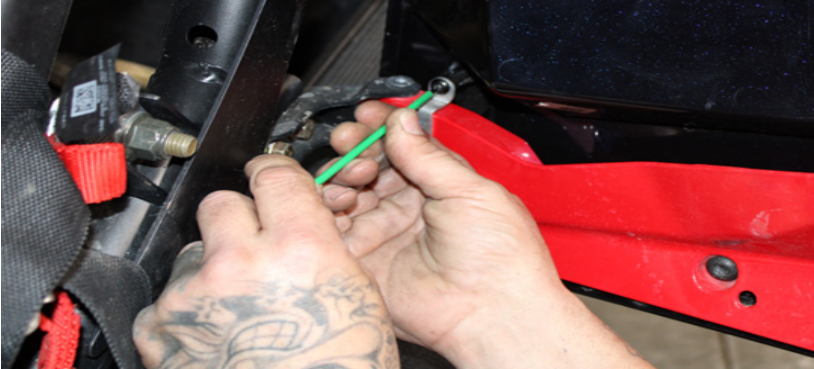
FIG 1 - Remove Door Strap with T25 Torx
