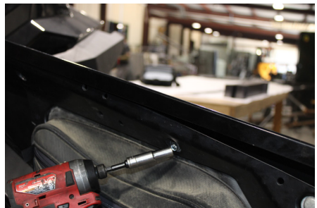
FIG 6 - Fasten Thumper Fab doors skins using 10mm socket
