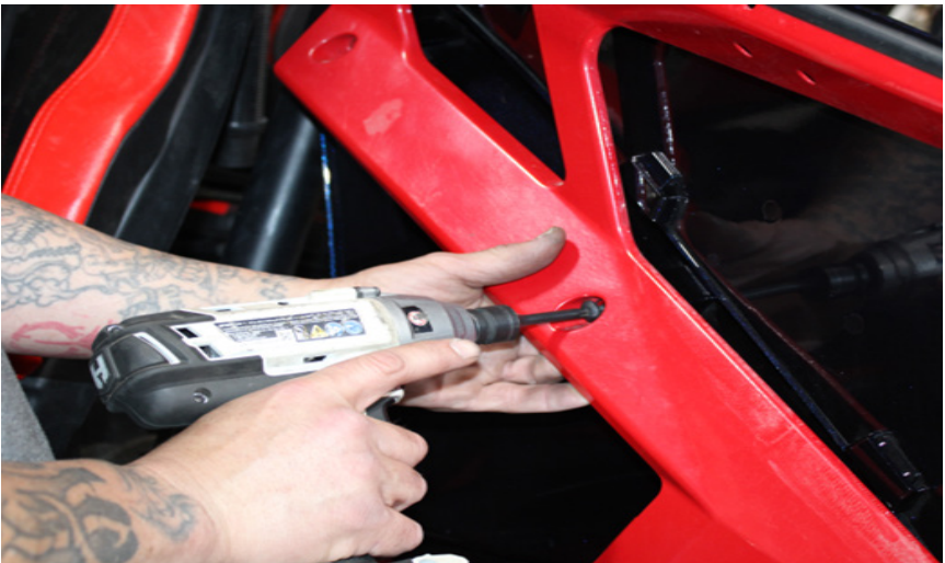
FIG 2 - Remove OEM doors skin using T40 Torx
