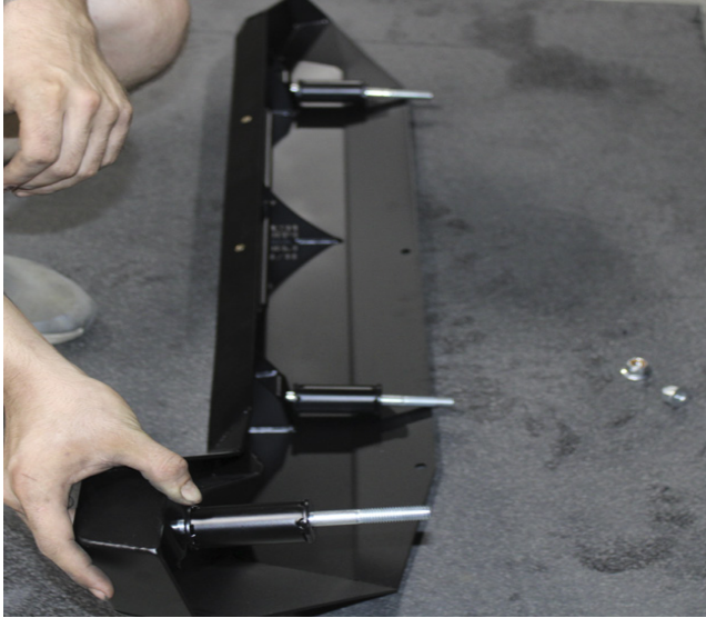
FIG 3 - Insert Hex Bolts (A) through rock slider and slide mount tubes (3) over Hex Bolts (A)
