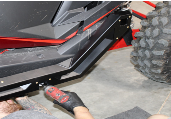
FIG 7 - Use a 19mm Socket and an 18mm Wrench to tighten mounting hardware
