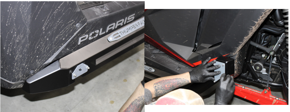
FIG 10 - Use a 9/64" Allen to fasten accent panels rock sliders
