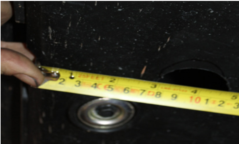
FIG 2 - Measure 4 inches from edge of skid plate to mark center of hole. Use 1.5" hole saw to drill out hole
