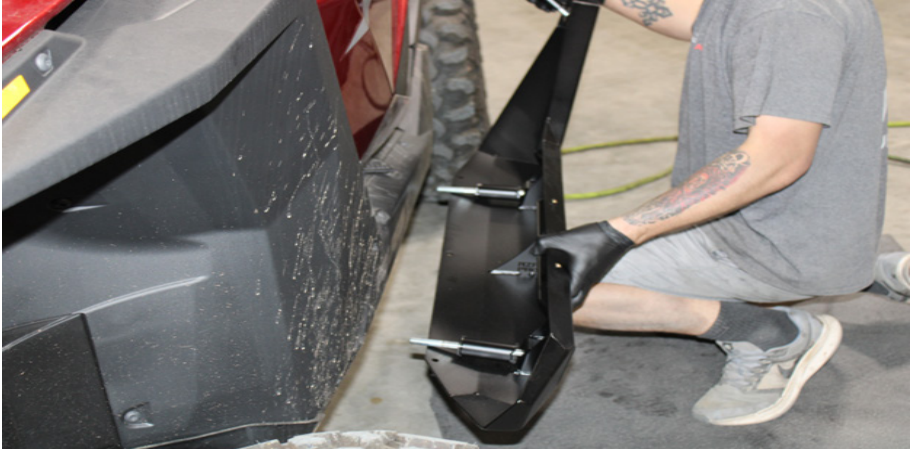
FIG 4 - Slide Mount Tubes (3) through provided holes in plastic and fit rock slider to unit
