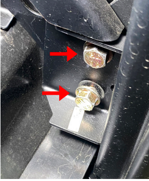
FIG 5 - 13mm Factory Bolts
