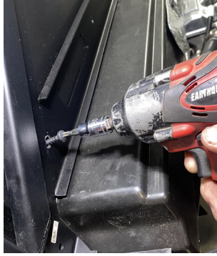
FIG 6 - T-25 Torx Factory Bolts
