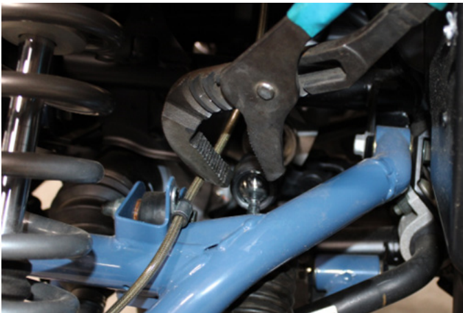
FIG 2 - Loosen inner tie rod using Crescent Wrench or Channel Locks and fully remove Tie Rod
