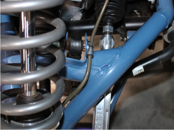
FIG 5 - Thread Jam Nut and Billet Tie Rod onto Inner Tie Rod
