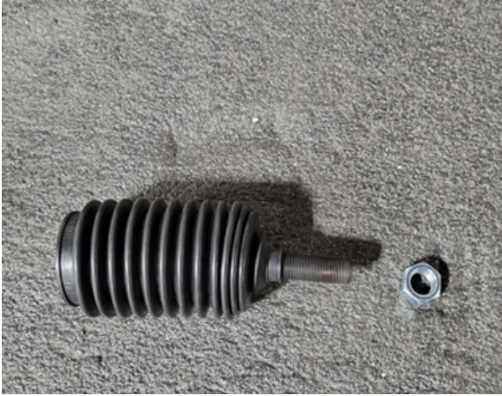
FIG 3 - Slide the Steering Boot over the Kryptonite Inner Tie Rod End
