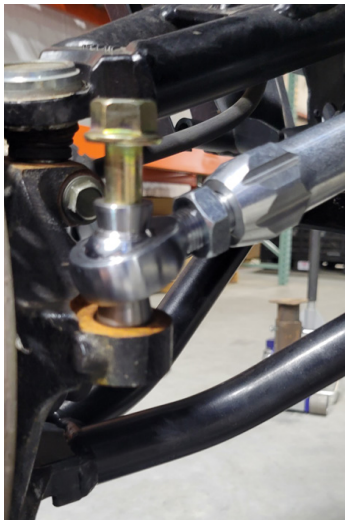
FIG 8 - Tighten Heim (3) to knuckle using 3/4" Socket and 3/4" Wrench
