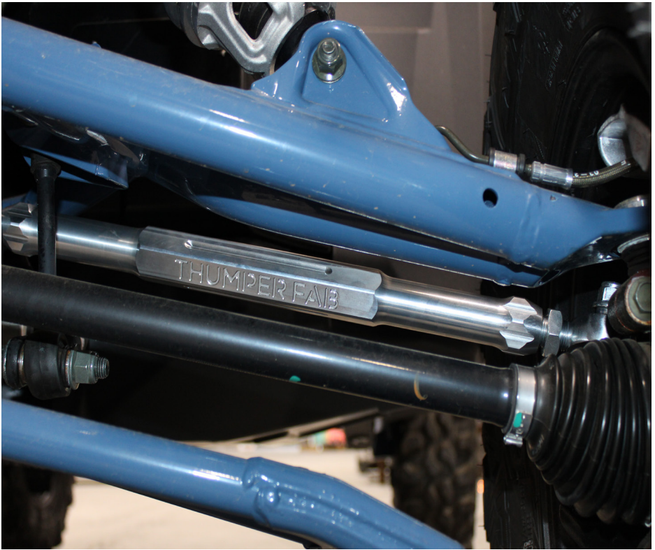
FIG 9 - Adjust Toe as needed and tighten Jam Nuts using a Crescent Wrench
