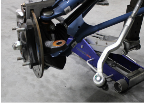
FIG 1 - Disconnect outer tie rod from knuckle using 18mm Socket
