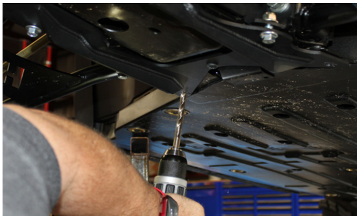
FIG 5 - Use 13/32" Drill Bit to Drill Holes in Factory Frame
