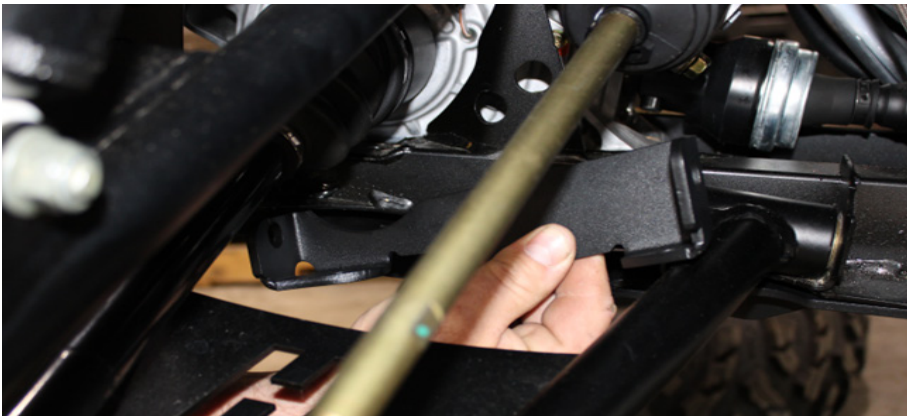
FIG 2 - Use A-arm Factory Bolts to Hold Middle Stiffener in place
