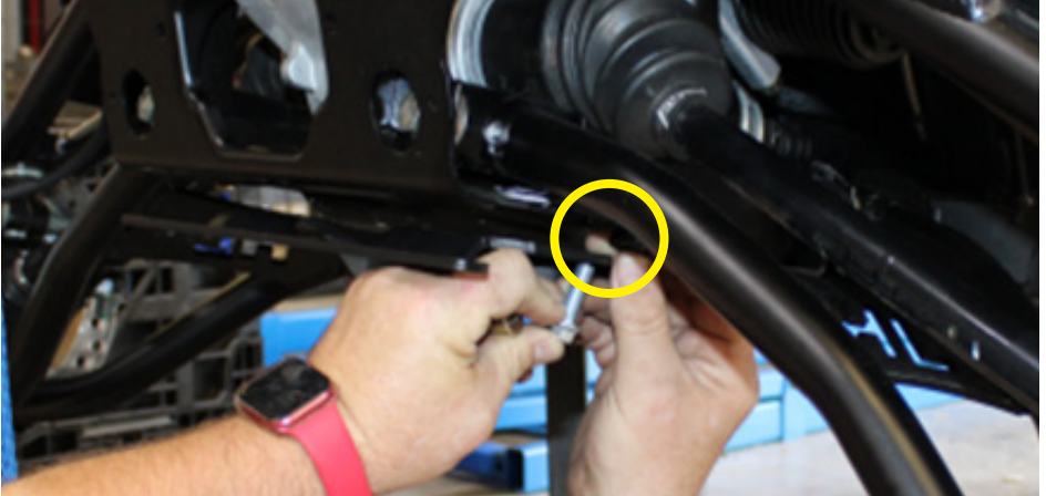
FIG 3 - Install Spacers (A) between Frame and Main Plate (1) using 15mm Wrench & 15mm Socket Finger Tighten
