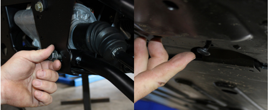
FIG 1 - Remove Tires, Front Bumper, Lower A-arm Bolts
