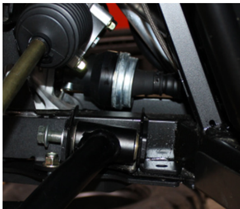
FIG 6 - Slightly Remove Factory A-arm Bolt
