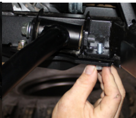
FIG 7 - Loosely install Bolt & Nut 15mm Wrench & 15mm Socket
