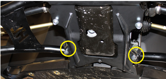
FIG 4 - Using 15mm Wrench & 15mm Socket Loosely attach Main Plate (1) to Frame
