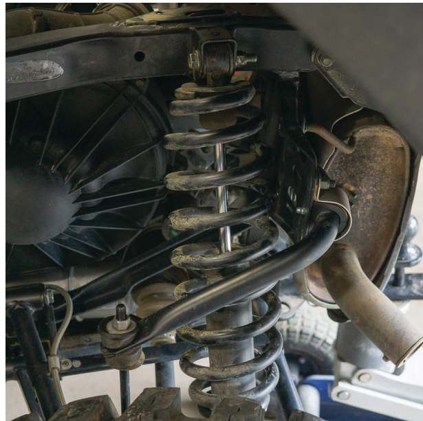
Fig. 6: Remove the upper shock hardware.
