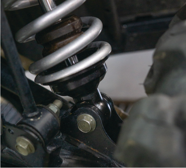
Fig. 3: Install the shock's lower mount.
