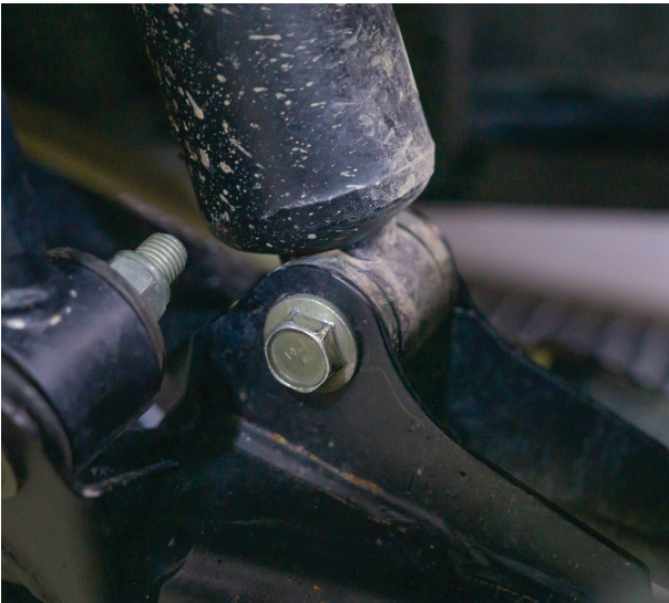
Fig. 1: Detach the lower shock hardware.
