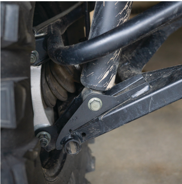
Fig. 5: Detach the lower shock hardware.
