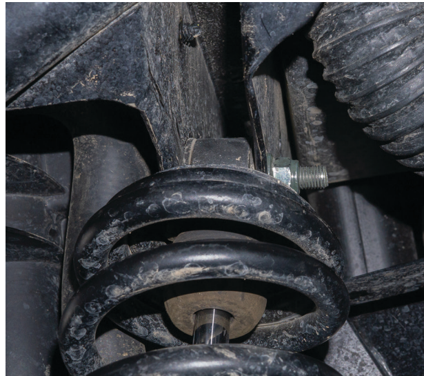
Fig. 2: Remove the upper shock hardware.
